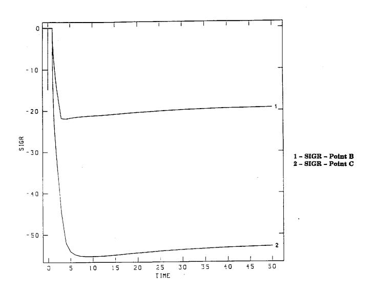
Figure 7-2. Radial Stresses - Case B.
